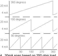
\*4...20mA span based on 250 ohm load
