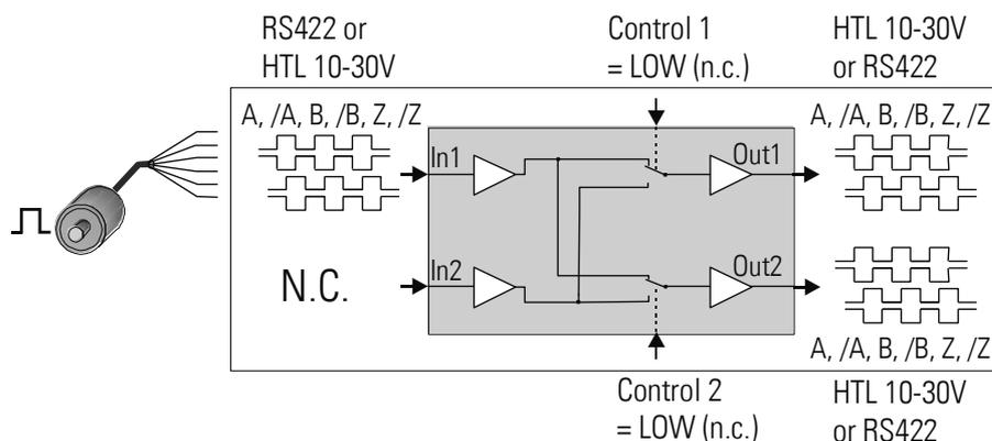
Input 1 is used as encoder input, and Input 2 remains unconnected. The input can be set to either symmetric (differential) format using A, /A, B, /B, Z, /Z channels, or to asymmetric (single-ended) format using A, B, Z channels only. Acceptable input levels are RS422, TTL and HTL 10 ... 30 V.
