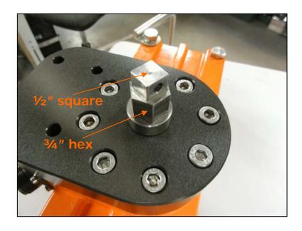
Once the retaining pin has been removed the squex can still be operated By using either a 3/4" spanner or a 1/2" spanner
