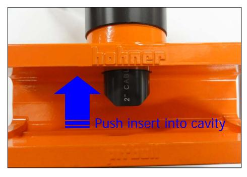
Push the selected insert into the cavity in the centre of the upper wall of the channel The tip of the 'squex' and each insert contain magnets to help hold one to the other Rotate the 'squex' until it mates with the insert; the insert should now be held in place
