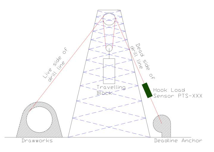
The above diagram is an overview of the positioning of the sensor
