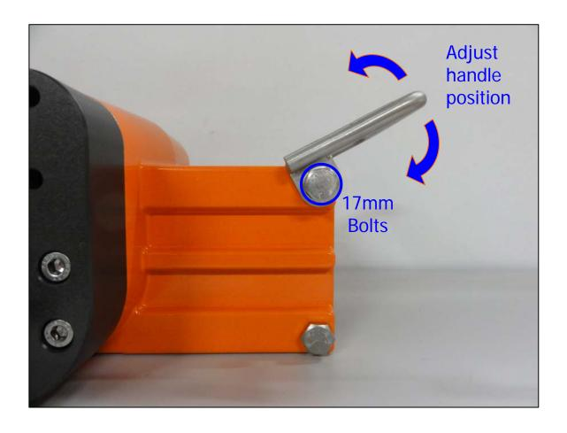
Before installing the hookload sensor it is important to lock the handle into position.
