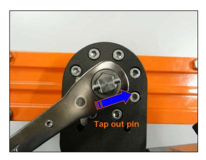
If the ratchet becomes damaged it can be removed by tapping out the retaining pin
