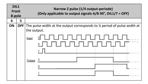
In this operation mode, only division ratios may be used, which together with the A/B divisor deliver clear and completely results. A division with rest causes that the Z pulse at the output can fluctuate around an input or output period.
