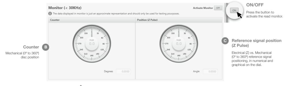
The PR90 encoder can be monitored with frequencies below 30 KHz (30.000 PPS).
