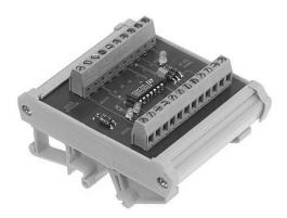
This interface module generates two additional static rotation direction signals (V, R) from the two output signals A, B phase-shifted by 900 of an incremental encoder.
