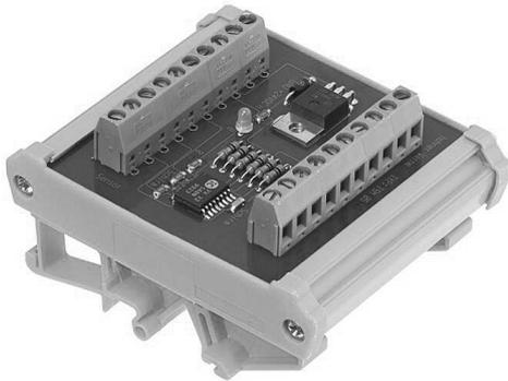
This interface module generates from the 24V signals A, B, 0 of an incremental encoder the 24V push-pull signals A, B, 0/AN, BN, 0N.
