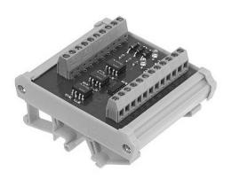
This interface module converts the 24V signals A, B, 0 of an incremental encoder into signals according to specification RS 422/485 (A, B, 0/AN, BN, 0N)
