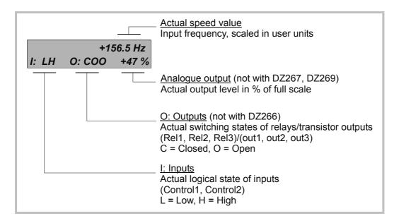
The "Display Menu" allows free scaling of the speed measuring values and the speed-related parameters to any kind of engineering units.
