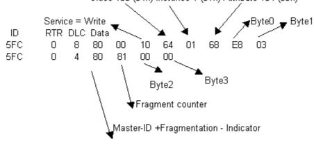
Set Measuring Range to 100.000 = 00 01 86 A0 h (Lowbyte is transmitted first!)
