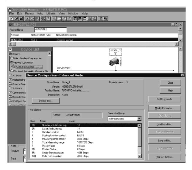
Pushing the "Save to device"-button the edited parameters will be transmitted to the encoder. Notice that all the transmitted values will be lost by switching off and switching on because the values are saved in the RAM of the encoder.
