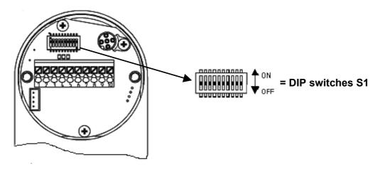
⇒ The DIP switches are accessible after bus terminal box has been drawn off.
